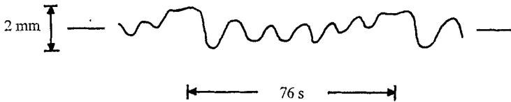
FIGURE 4. Wave form observed at probe location indicated in figure 3. Fundamental period ( 2\pi/\omega_0 ) is 76 s.
